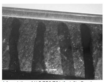
A formulation of ALB/PPS/ES1 (far left) offered the best results compared to 3 other formulations of alcohol ethoxylate/anionic based systems that were tested.
